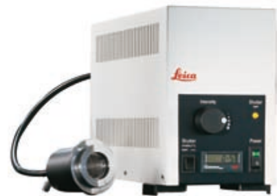
Leica EL6000 external light source with high-speed shutter for fluorescence excitation.
