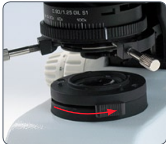
Close the Koehler field diaphragm
