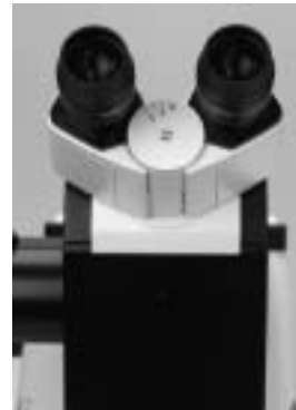
Fig. 22: Siedentopf tube with interpupillary distance adjustment
