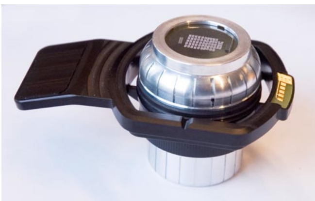
Fig 2. Special holder to support the polished metallurgical mounts up to 1 ¼ inch.
