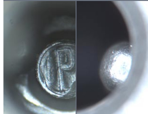
Detail of an injection nozzle – on the left: with Leica LED3000 NVI™, on the right with conventional ring illuminator
