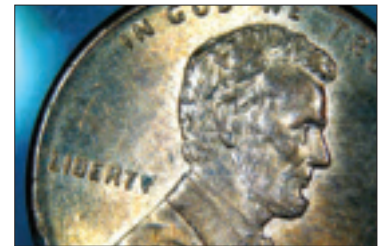
Stage 3 incident light: the lower two LEDs light finely structured objects from a low level, increasing contrast.
