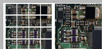
Real-time stitching can generate mosaic images while moving the stage
