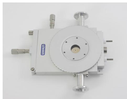
*The THMS350V heating and freezing vacuum stage*
