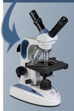
The EXM-151-T features a dual-view teaching head, mechanical stage, a 100xR oil objective, and an N.A. 1.25 Abbe condenser
