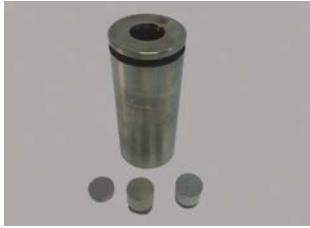
Mould assembly, with intermediate ram
