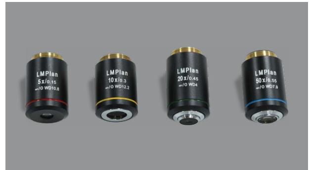
IOS LWD U-PLAN MET (5x, 10x, 20x, 50x) Objectives. 100x is optional
