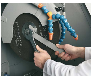
Easy Exchange of Cut Off Wheel
