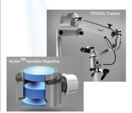
The PRIMA TRAINER comes with a clip-on objective protector to shield the optics from spray back and debris. Floor, wall, mobile, ceiling, and traditional table mounting options are available, as well as an extra long suspension arm (provi dirg an additional ~250mm) for further removed mounting orientations. A host of eyepiece and objective options are available to further customize the PRIMA TRAINER.
